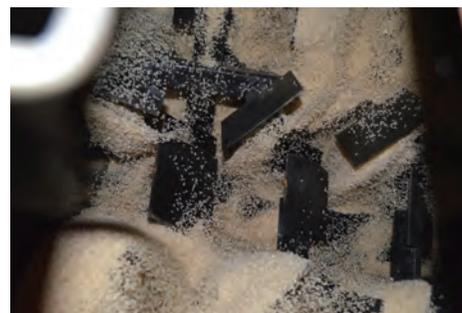
**Figure 5.2.** Rice blending inside the Forberg fluidised bed blender
