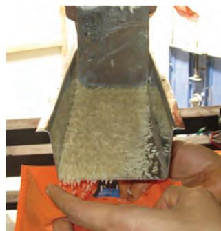
**Figure 3.3.** Calibration of dosing equipment is very important for continuous blending. See the Annexes for an example calibration record keeping format
