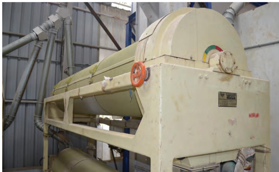
**Figure A11.** Example blending setup – rice length grader adapted for use as a horizontal blender
