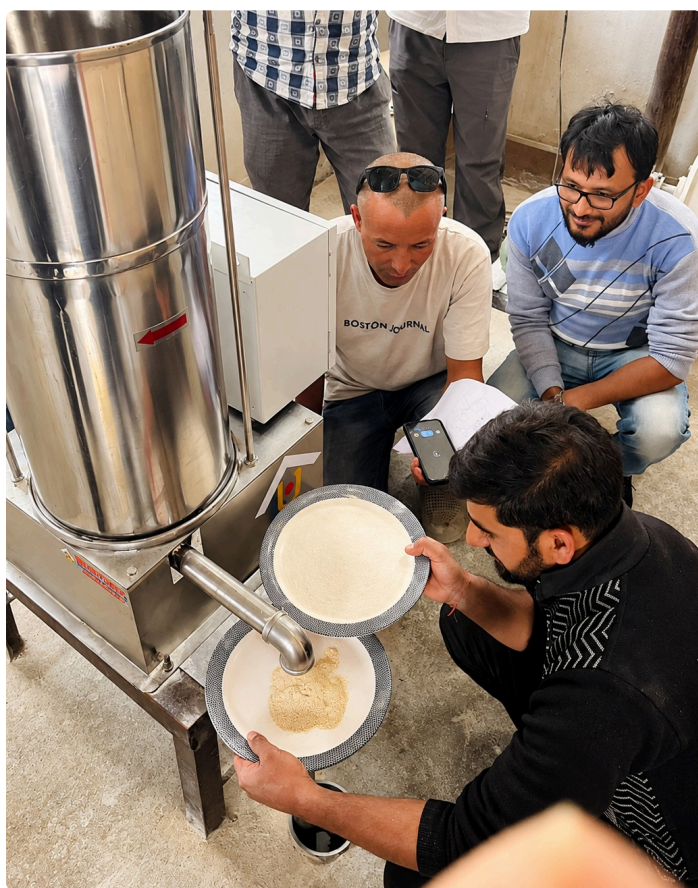
Millers checking pre-blend discharge from microfeeder (calibration) during on-site training.
